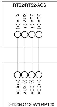
NOTE: If polarity of Acc. (+) and Acc. (—) are reversed, an Amber LED on sensor 2 of the duct smoke detector power board will exist indicating a trouble condition.
